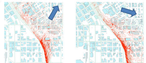
Figure: Downwind dispersion patterns of vehicular emissions from I-5 in downtown Seattle. Predictions are from the QUIC model. Dark red indicates higher concentrations. Blue arrows indicate average wind direction.
