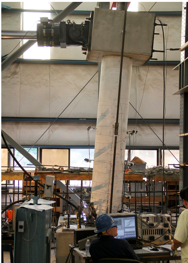
Figure 1: Reinforced concrete column with HSS subjected to lateral loads.
