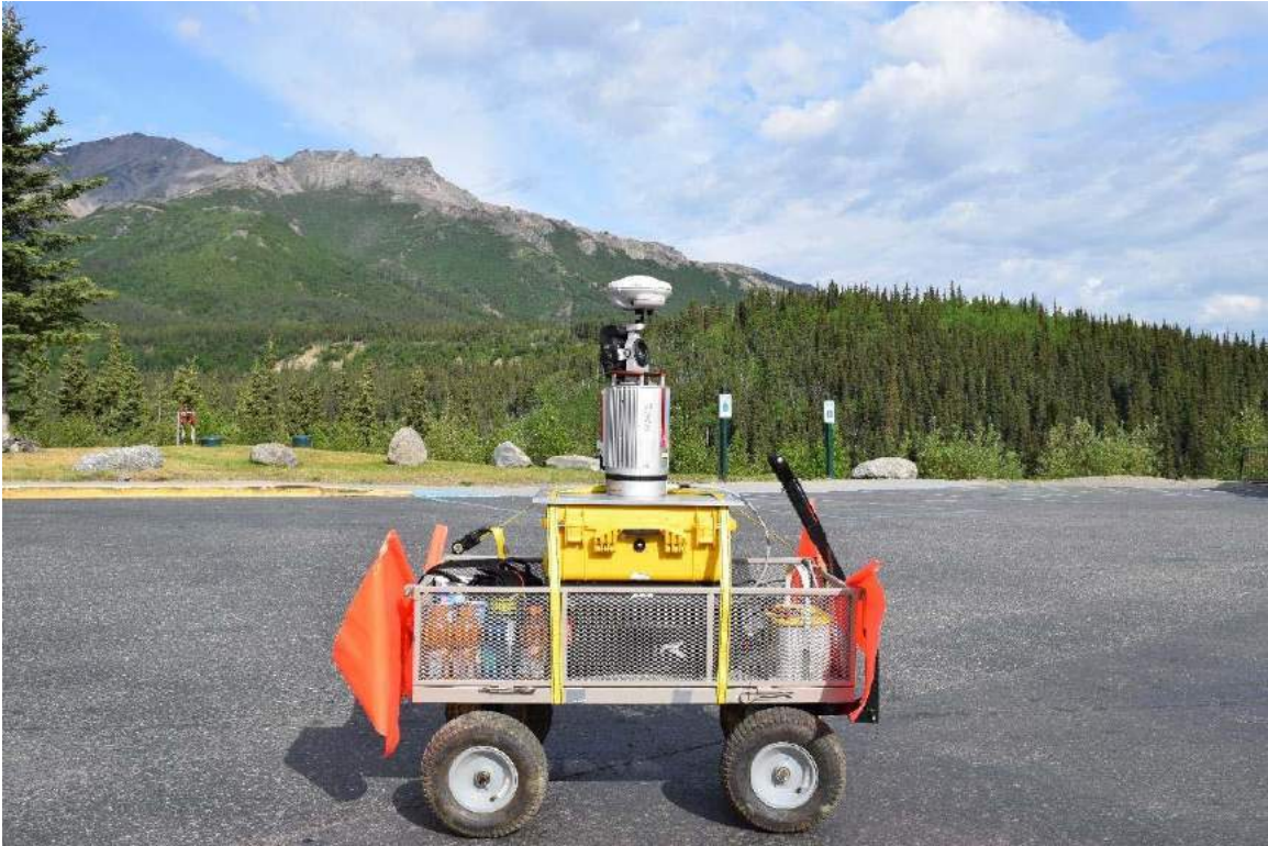
Figure 4.4 - TLS survey platform
