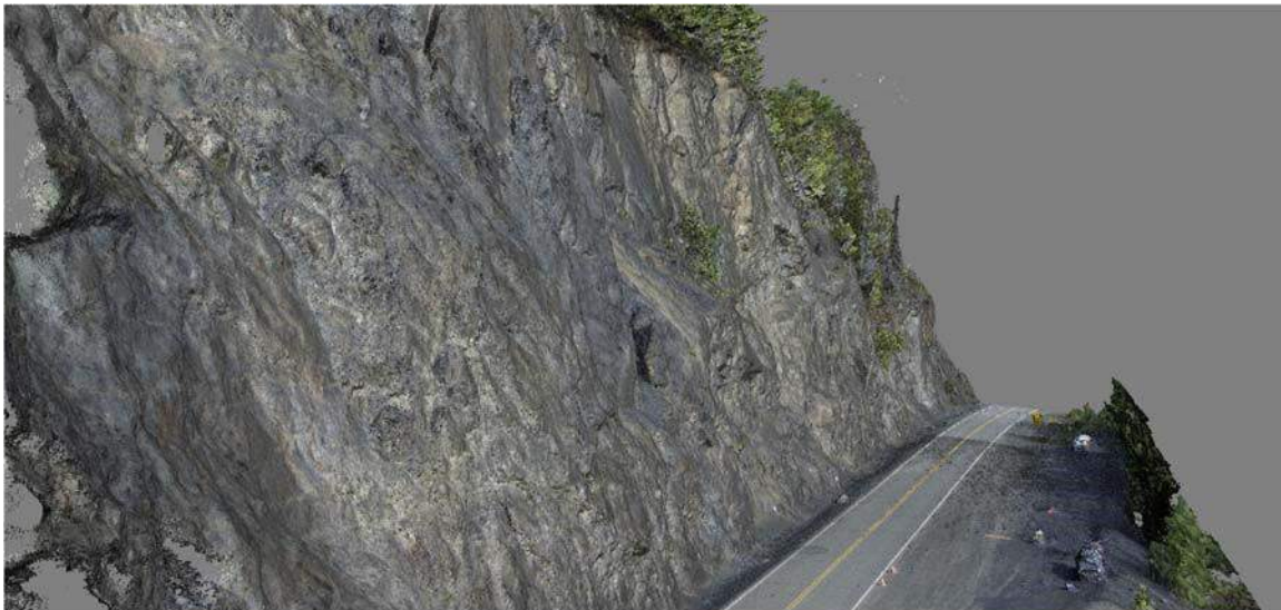
Figure 5.1 - DSM model example from UAS imagery and SfM processing
