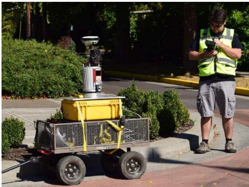
**Figure 3.3** STLS mobile wagon set-up for stop-and-go scanning of the intersection.
