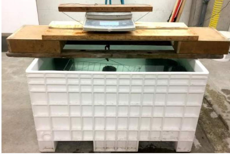
Figure 4.2: Water bath for submerging specimens for porosity testing.
