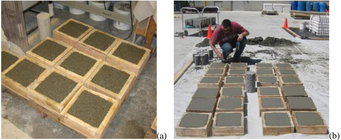
Figure 4.1: a) Cast PC slabs and b) cast PCC slabs and final finishing.
