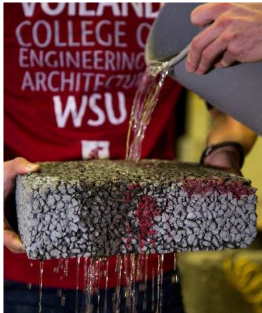
Figure 1.1: Pervious concrete allows infiltration of runoff through the pavement surface.
