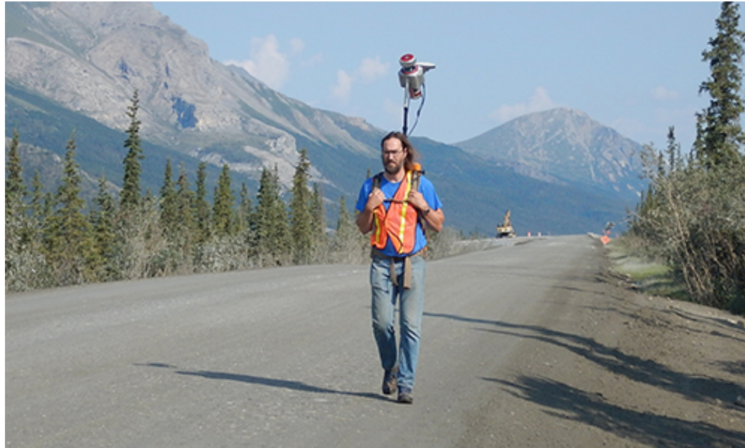
Collaborator Dr. Ronald Daanen walking with the backpack-mounted LiDAR along the old Dalton Highway embankment, July 2018 (photography by M. Darrow).
