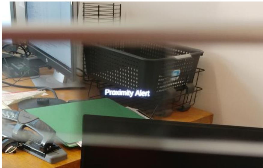
Figure 6: Snapshot of view to worker with digital warning overlaid on real world content
