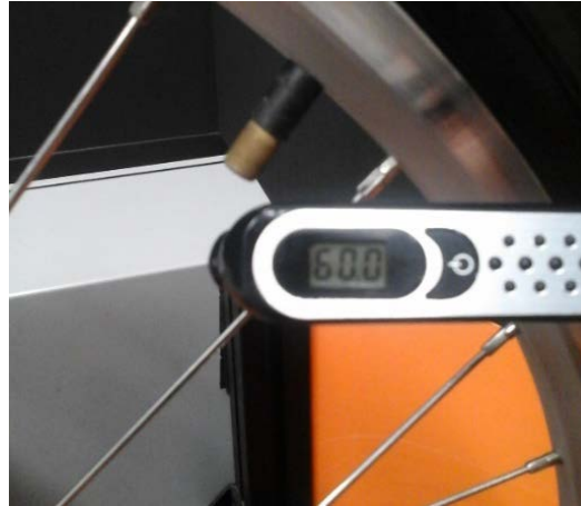
FIGURE 8 Digital tire pressure gauge during tire pressure analysis
