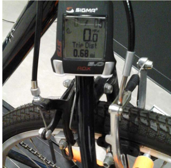
FIGURE 2 Bicycle computer used to collect the physical speed of the wheel.
