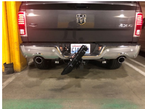
Figure 1 RCM 411 Sensors on Maintenance Truck of WSDOT
