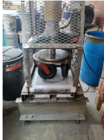
Three-wheel polisher to simulate the effect of traffic loading during winter treatment operations
