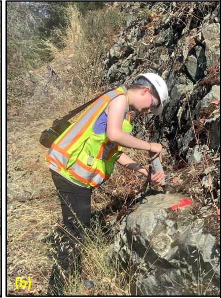
Acquisition of Schmidt Hammer (SH) readings at sites in (a) Alaska and (b) Oregon (photographs by M. Darrow).
