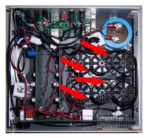
4. The batteries are now loose. Dispose of them as directed. Carefully install new batteries by following these steps in reverse. Be sure to note the positive and negative terminals on the batteries, the labels are molded into the plastic. The RED wire connects to POSITIVE (+) and the BLACK wire connects to NEGATIVE (-).
