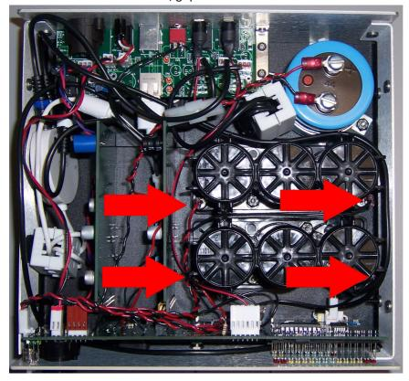
3. Remove the 4 hex nuts holding in the batteries. The hex nuts have nylon inserts, so it will be necessary to hold the screw from the bottom using a Phillips-head screwdriver.
