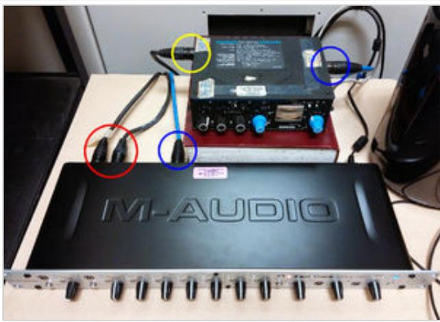
Connections. Head-mounted mics connected in channels 1 and 2 (circled in red), amp connected to channel 5 (circled in blue), stand mic connected to amp (circled in yellow)
