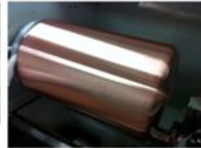
EF copper after machining
