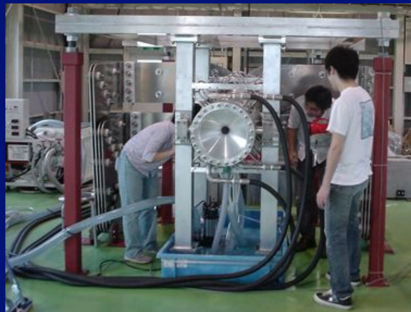
Target/Horn magnet – test setup Must handle pulses of 100s of kA
