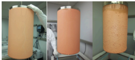
Inspection of EF copper on mandrels
