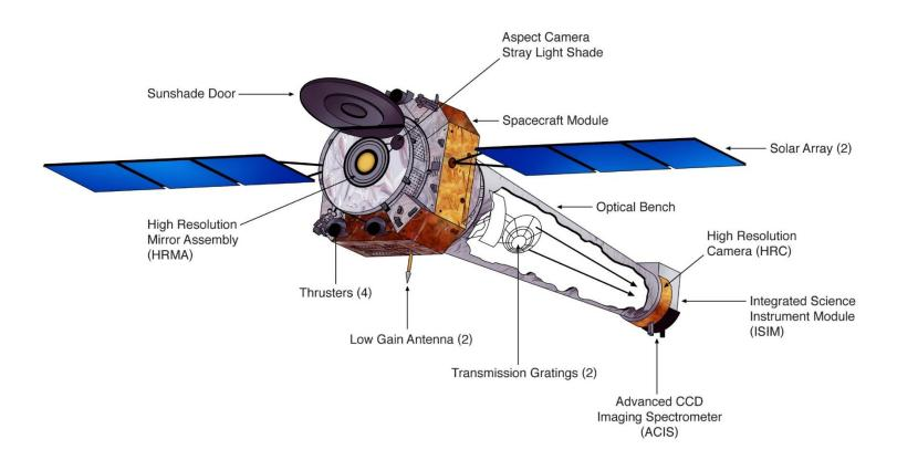
The most advanced X-ray telescope in use today Almost 14 meters in length Operates in the 0.06-10 keV range Highly eccentric 64 hour orbit for long exposures
