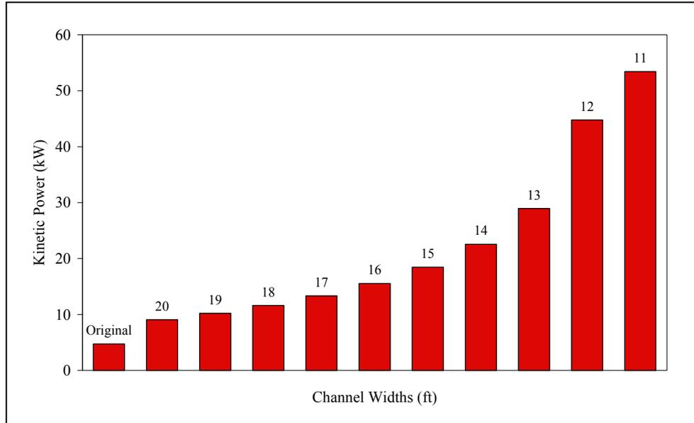
Figure 7.2: Kinetic Energy Resource for Check 5 at Various Channel Widths
