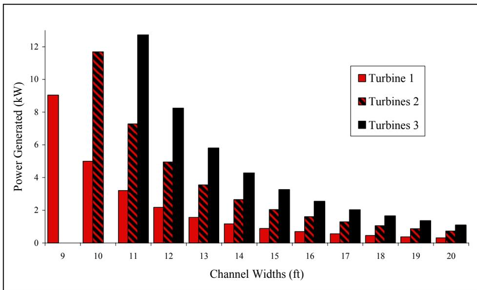
Figure 6.6: Power Generation for a 10 kW Turbine at Various Channel Widths
