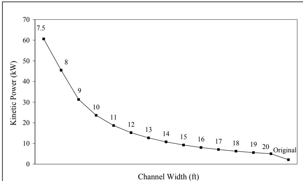
Figure 6.2: Kinetic Power Resource at Check 2 for Various Channel Widths
