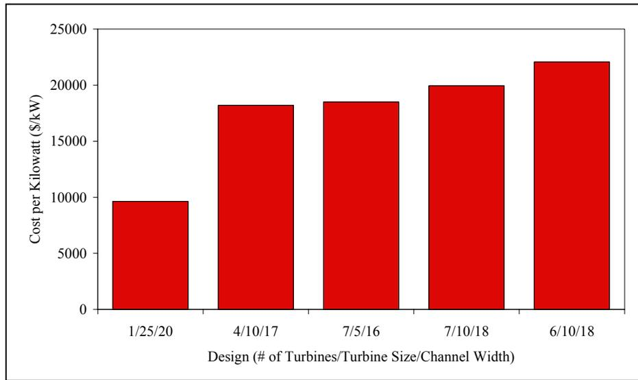
Figure 7.6: Top Five Low-Cost Design Options for Check 5
