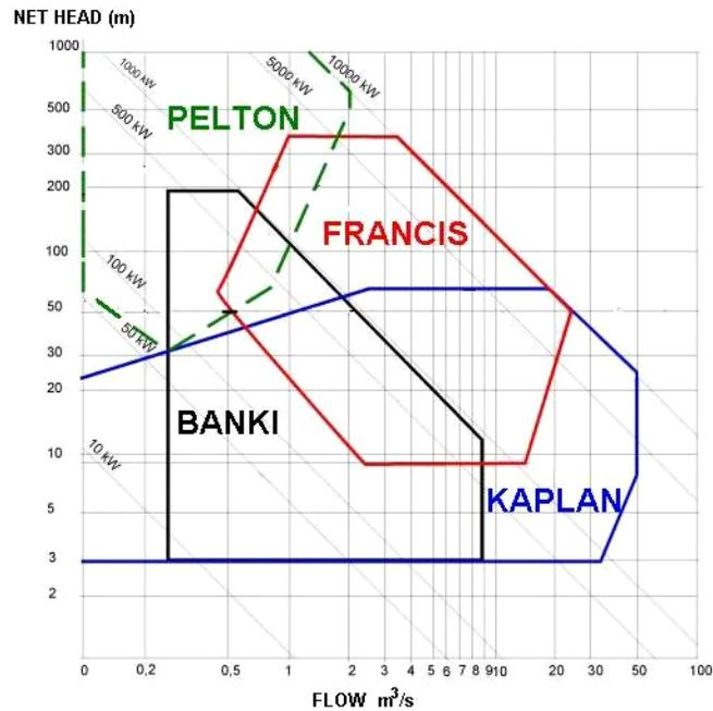
Figure 6.11: Hydropower Turbine Selection Graph [26]
