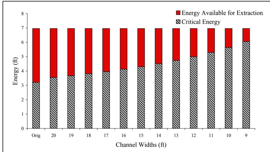
Figure 6.4: Difference between Channel Specific Energy and Critical Specific Energy for Check 2
