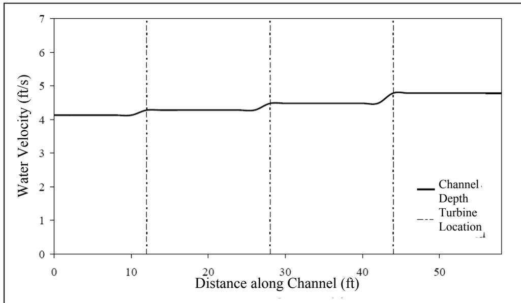
Figure 6.9: Approximate Change in Velocity in a Channel due to Power Extraction
