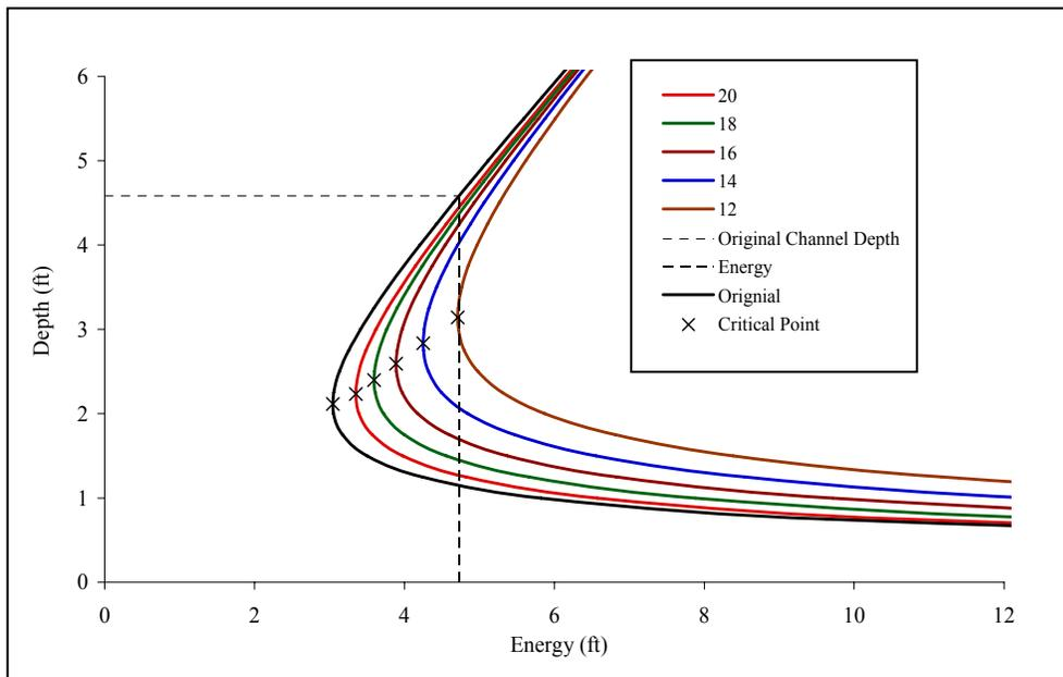
Figure 7.3: Sample of Specific Energy Curves at Various Channel Widths for Check 5
