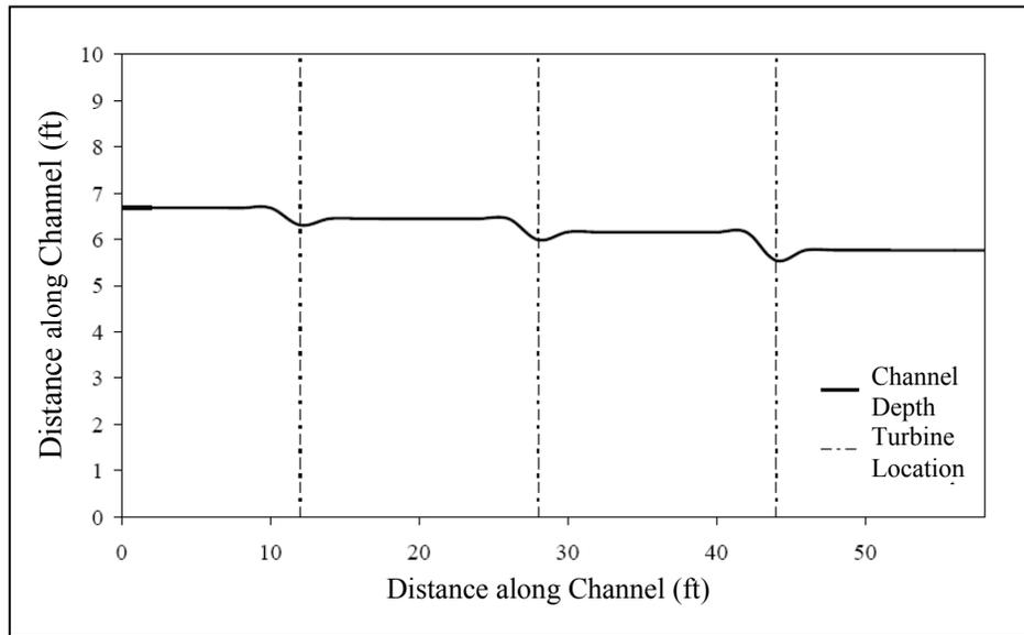
Figure 6.8: Example of Water Depth Profile with Power Extraction
