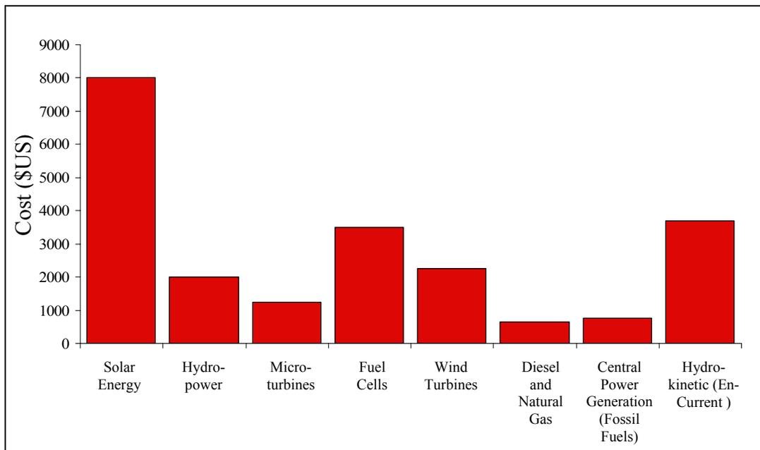
Figure 2.4: Average Cost per Installed Kilowatt for Various Energy Sources [11]
