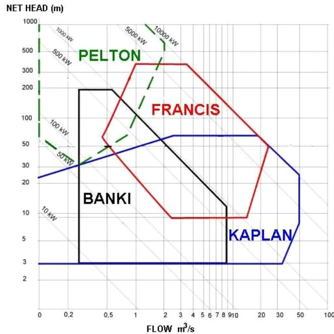
Figure 6.11: Hydropower Turbine Selection Graph [26]
