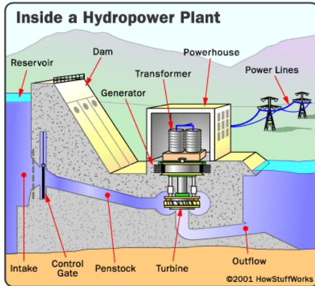
Figure 3.1: Typical Design of a Conventional Hydropower System [13]
