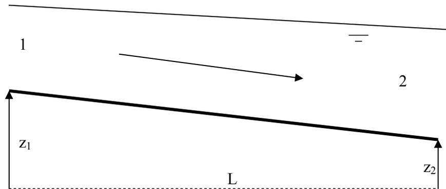
Figure 5.1: Diagram for Standard Step Method
