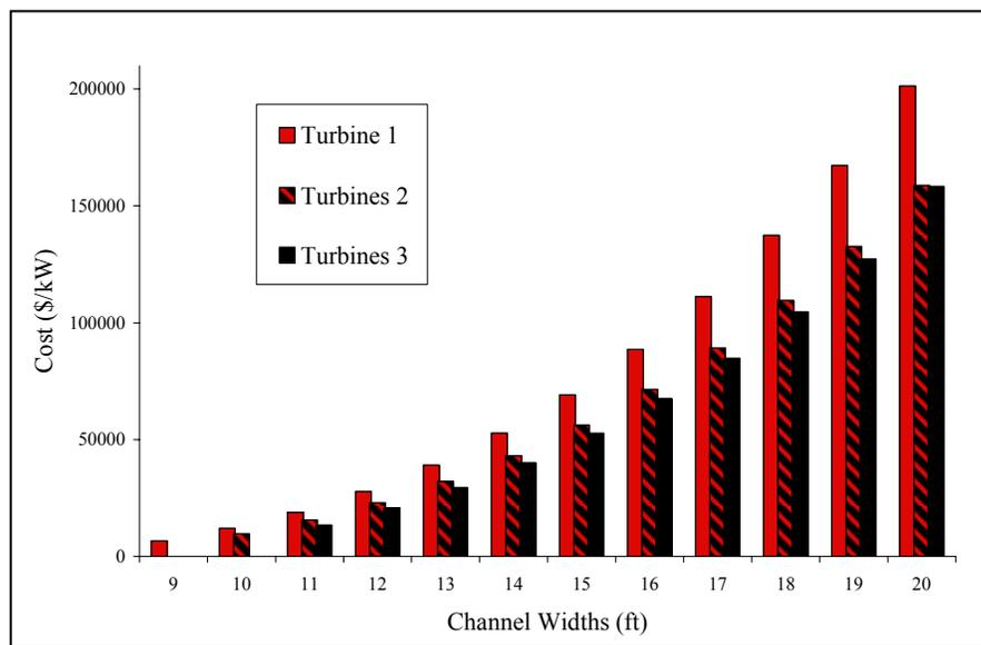
Figure 6.7: Cost per Kilowatt for a 10 kW Turbine at Various Channel Widths
