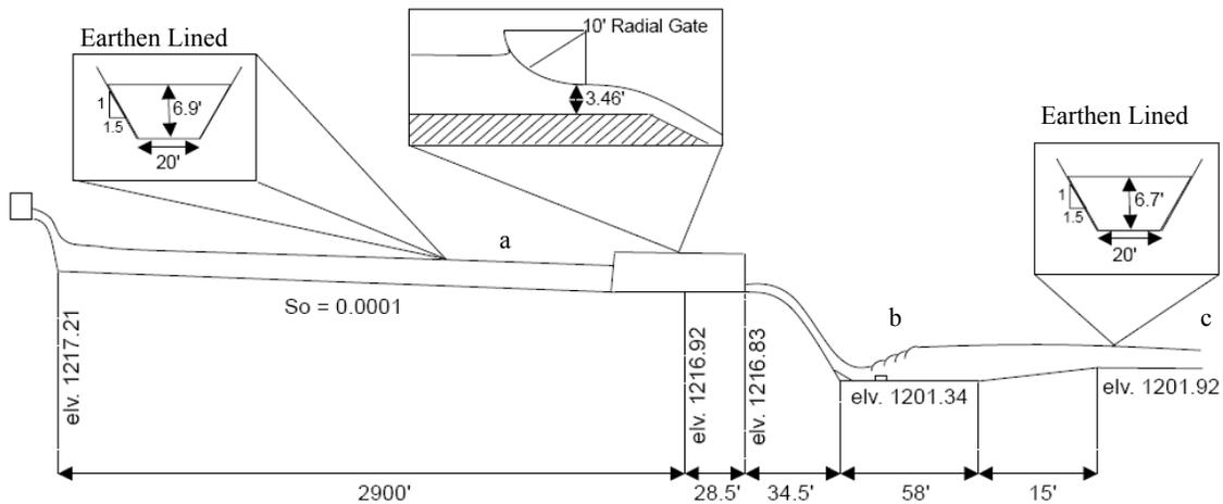
Figure 4.4: Original Design of Check 2 on East Low Lateral 68
