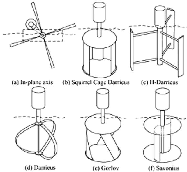
Figure 2.2: Examples of Hydrokinetic Turbine Designs [9]
