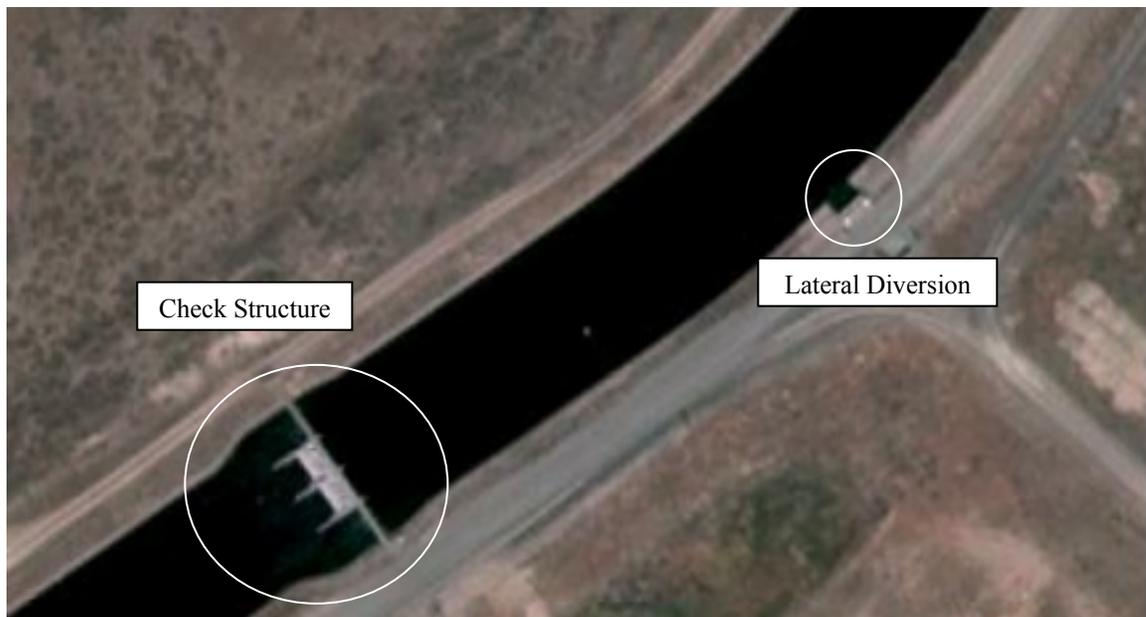
Figure 4.2: Aerial View of Check Structure and Lateral Diversion [16]
