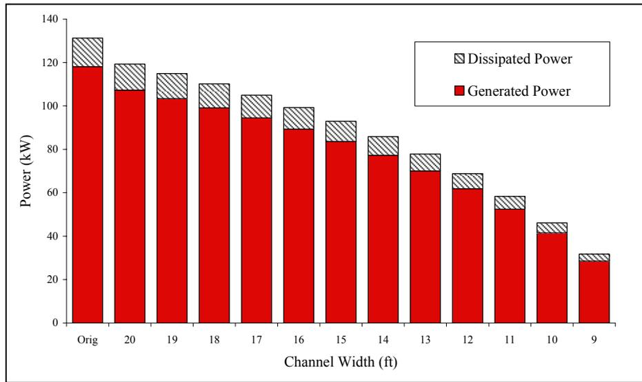
Figure 6.5: Expected Power that can be Extracted Based on Channel Width for Check 2
