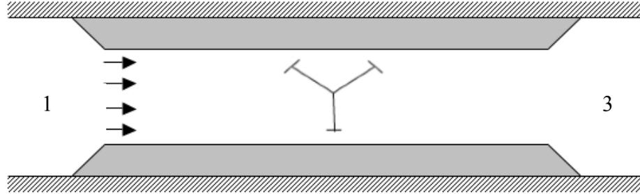
Figure 5.5: Channel Constriction with Turbine
