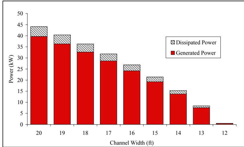
Figure 7.5: Expected Power that can be Extracted Based on Channel Width for Check 5
