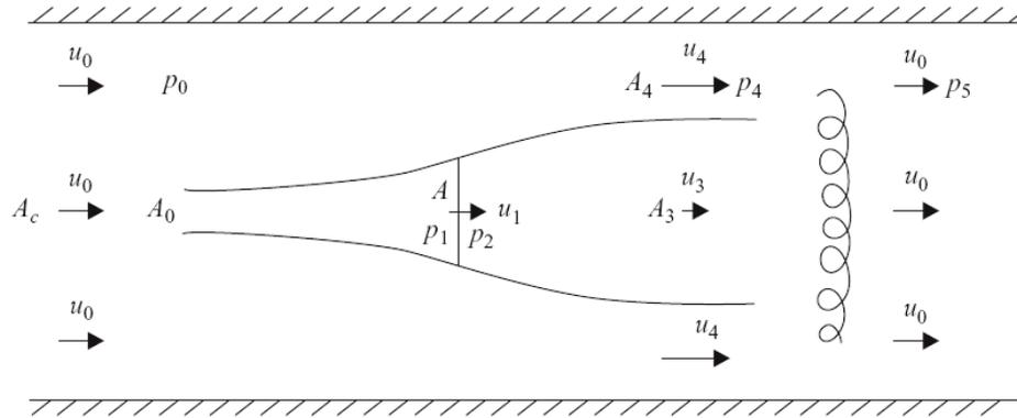
Figure 5.4: Definition Plan View Sketch of a Single Turbine in a Channel [24]
