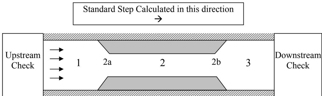
Figure 5.2: Sketch of Channel Constriction
