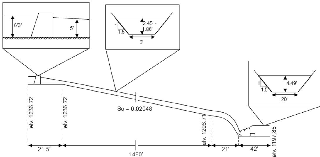
Figure 4.8: Sketch of “Cemetery” Check on East Low Lateral 29
