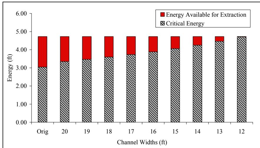
Figure 7.4: Difference between Channel Energy and Critical Energy for Check 5
