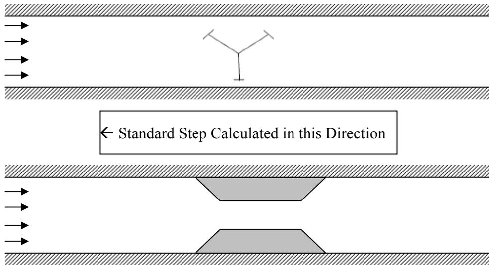
Figure 5.3: Sketch Turbine in Flow Replace by a Channel Constriction
