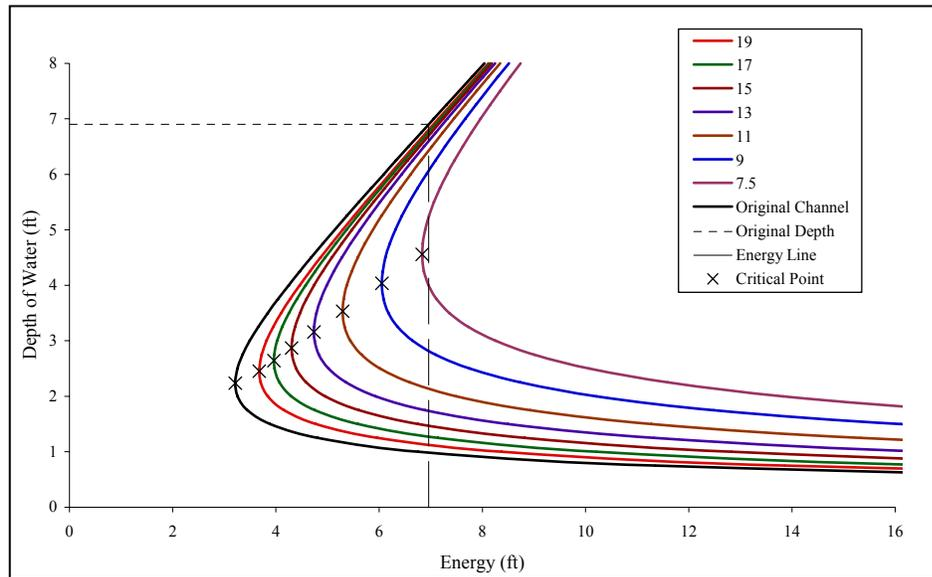
Figure 6.3: Sample of Specific Energy Curves at Various Channel Widths for Check 2
