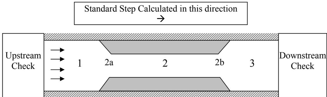
Figure 5.2: Sketch of Channel Constriction
