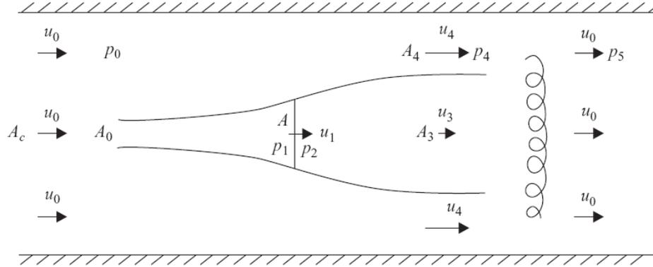
Definition sketch of a single turbine in a channel [24]
