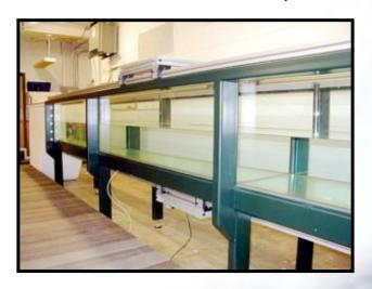
Wave-Current Flume: Experimental studies of tidal turbine wakes.
