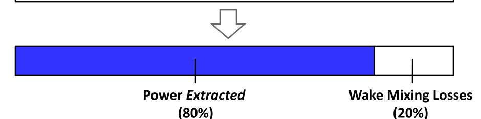
99% Dissipation Coefficient ( $\eta_d$ ) 1/3 Blockage Ratio ( $\varepsilon$ )
