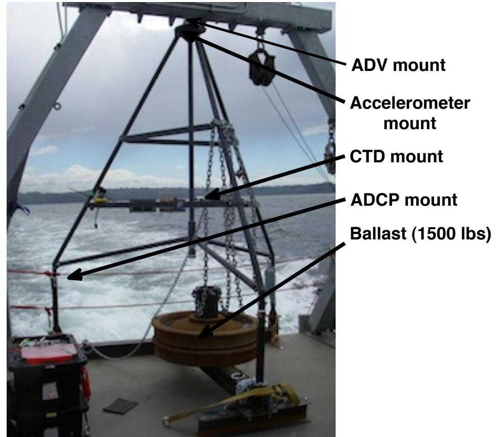
5 m tripod deployed in 22 m water depth
