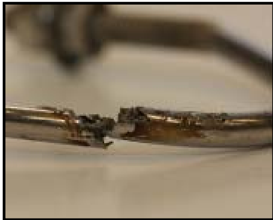
316 Stainless – Crevice Corrosion
