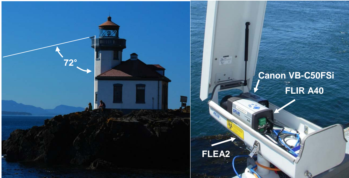
Figure 2.1 The mounting location and geometry for the cameras at Lime Kiln Park.
