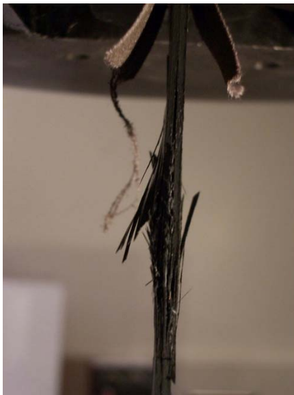
Figure 7-14: Pre-Preg Specimen T1, Seconds Before Final Fracture
