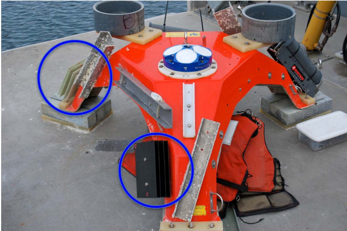
Figure 5-4: Panels Mounted on Sea Spider Prior to Initial Deployment
