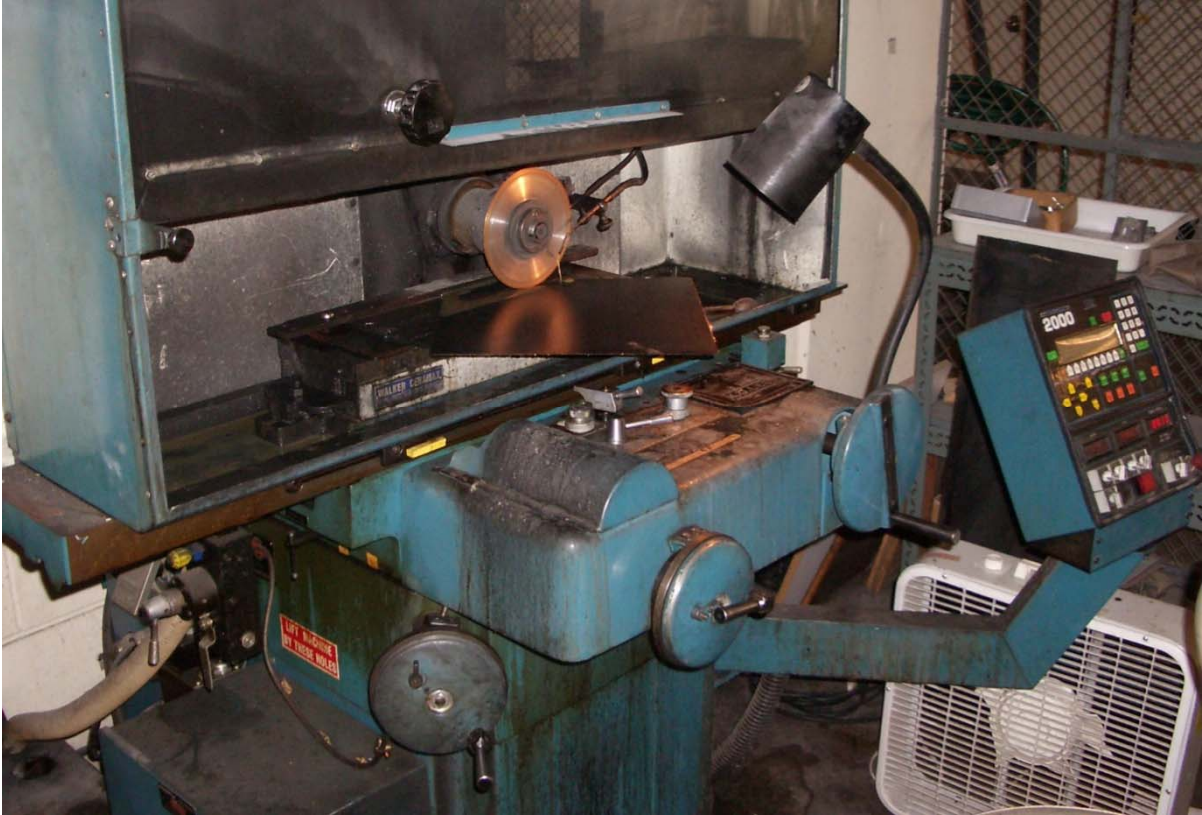
Figure 5-2: K.O. Lee Surface Grinder in the Process of Cutting a Pre-Preg Panel
