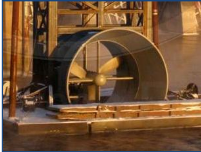
Figure 1.5 Hydro +TM shrouded horizontal axis turbine. Image corresponds to the deployment in front of the Lock and Dam No.2.
