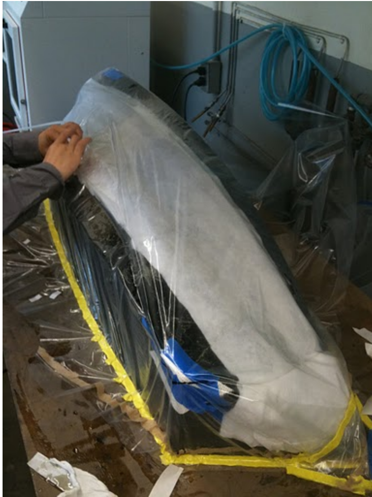
Figure 11: Completed Layup with Initial Covering
