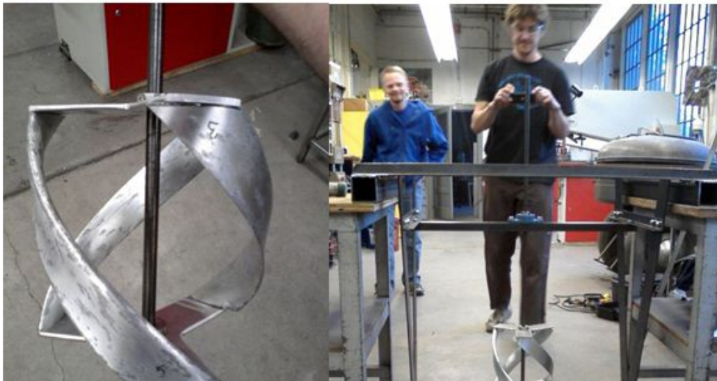
Figure 6: Turbine #1 constructed (left) and mounted in the gantry (right)
