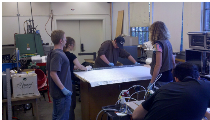
Figure 9: Cutting Fiberglass Layers
