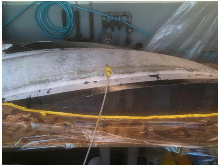
Figure 12: Vacuum Sealed Layup
