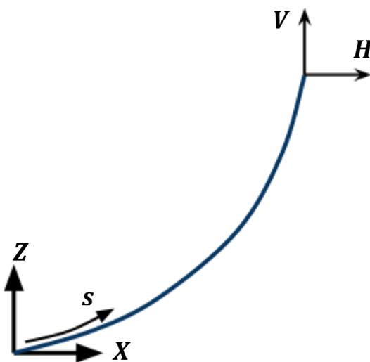
**Figure 4.1** Elastic catenary setup
