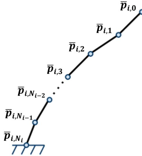
**Figure 2.3** Mooring line segments and nodes
