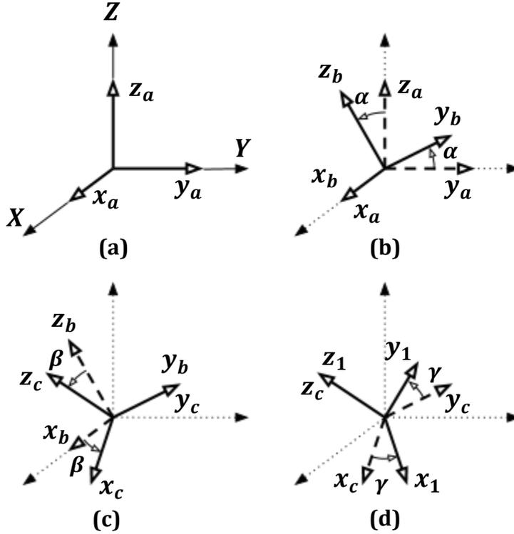
**Figure 2.2** Euler rotations of intermediate frames
