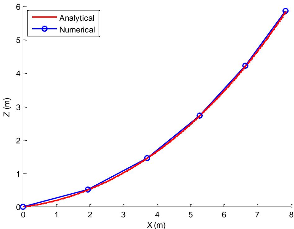
**Figure 4.2** Elastic catenary analytical and minimized solution using 5 line segments
