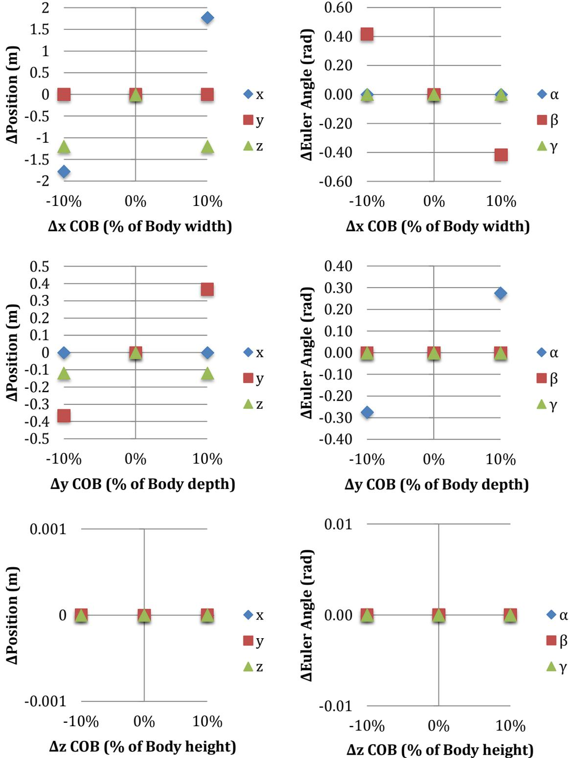
Figure 5.17 Change in body's position and Euler angles due to variation of body's COB
