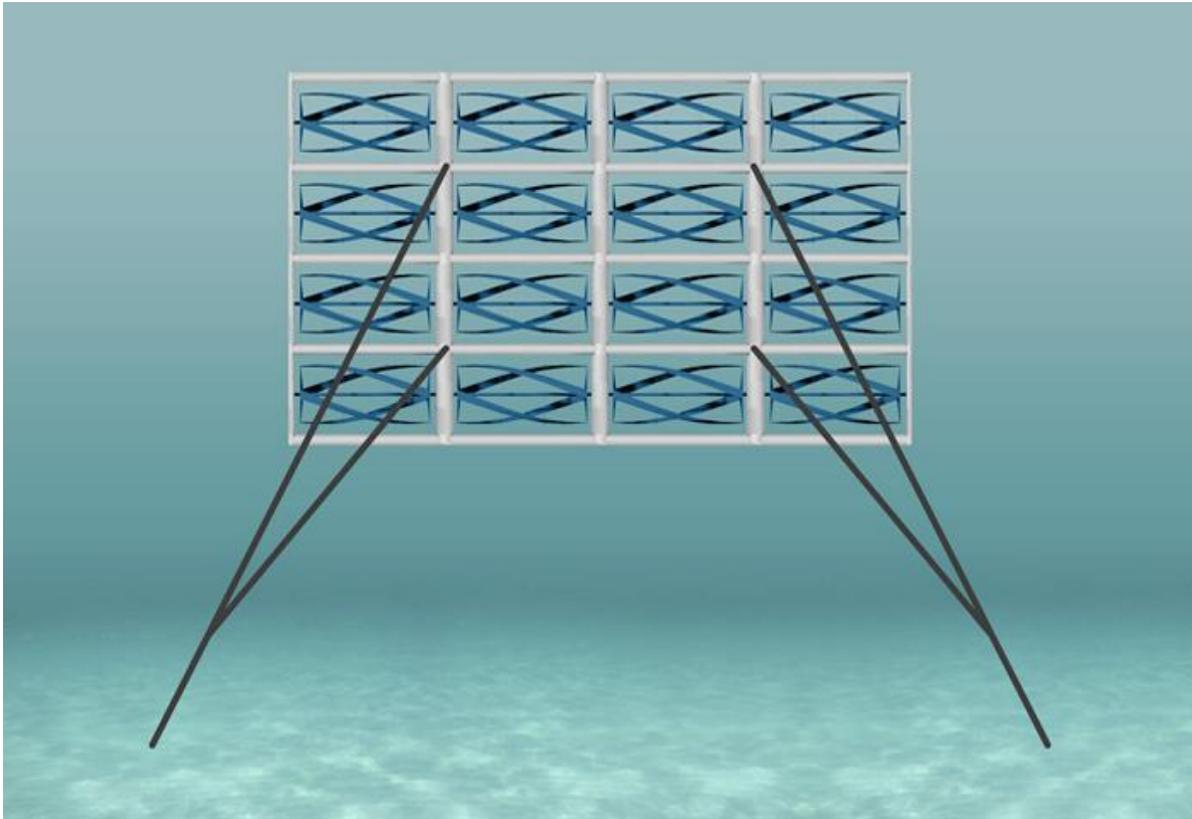
**Figure 1.1** Concept image of ORPC's OCGen™ system, submerged body and mooring line system example (1)
