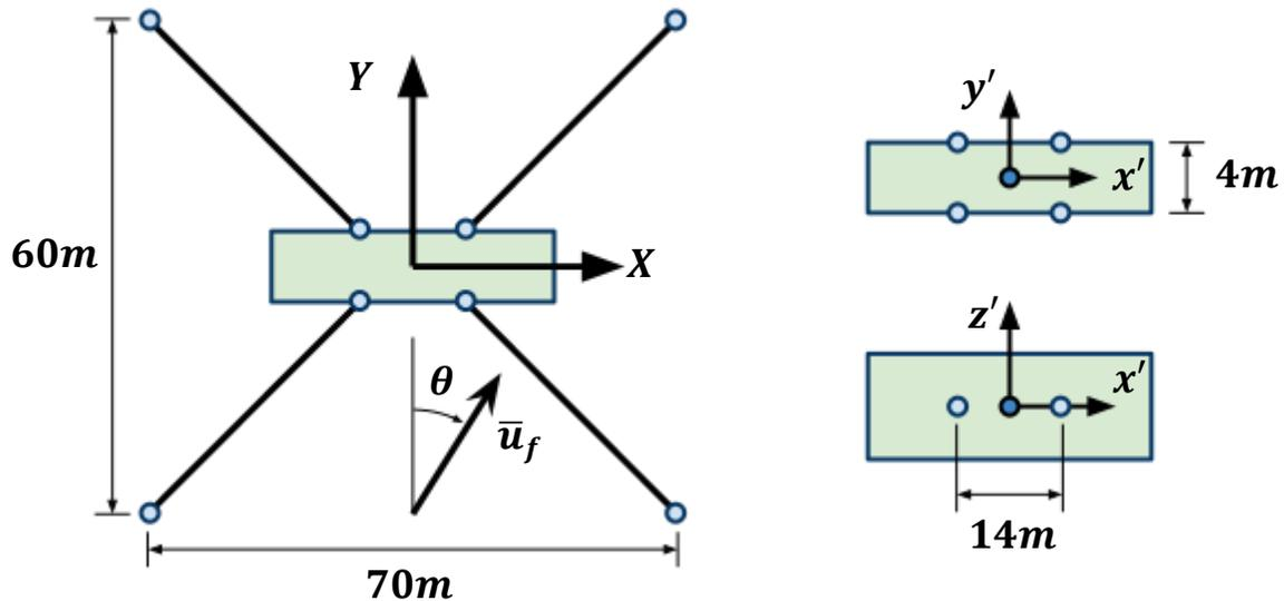
**(a)** Inertial frame and system setup, top view, showing mooring line ground attachment points and fluid velocity
