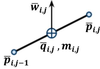
**Figure 3.1** Segment center of mass and net buoyant and gravity force
