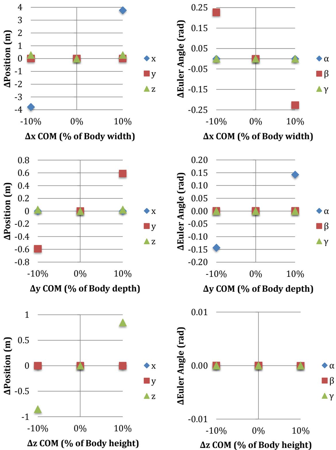
Figure 5.16 Change in body's position and Euler angles due to variation of body's COM
