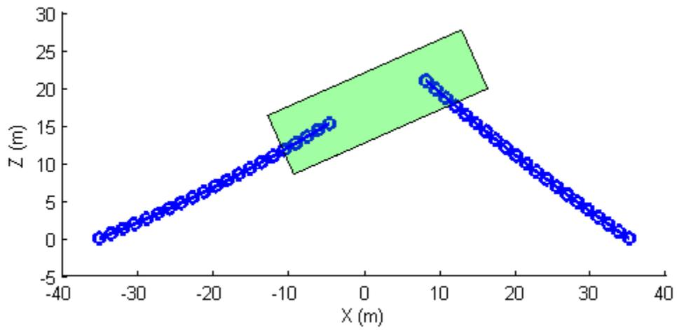
**Figure 5.19** Equilibrium position due to  $\Delta x$  variation in body's COB
