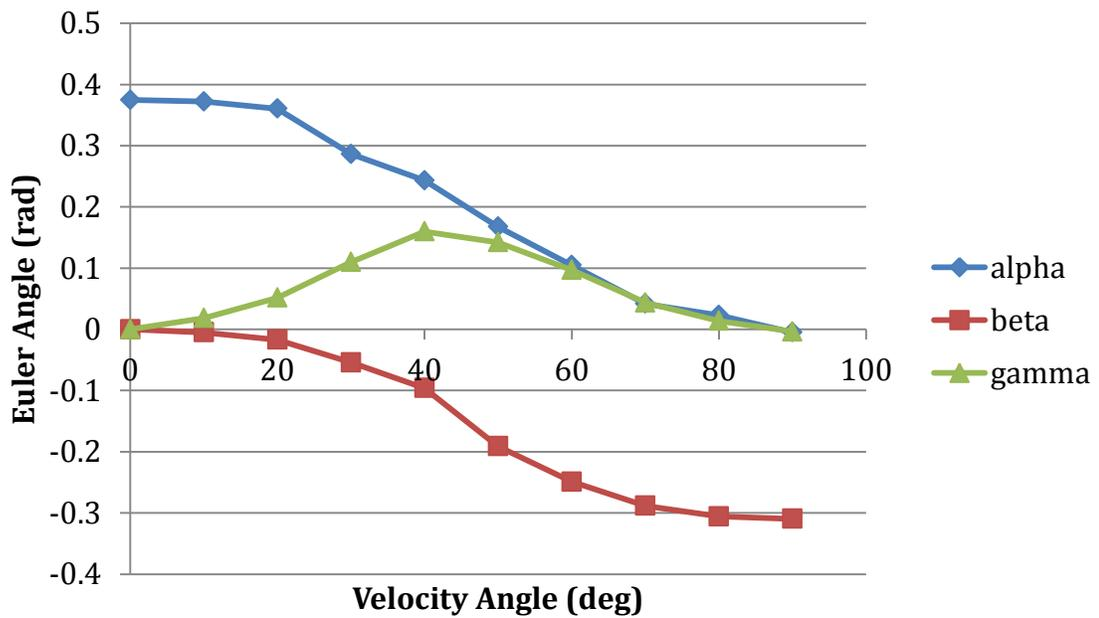
Figure 5.13 Body's Euler angles versus velocity angle
