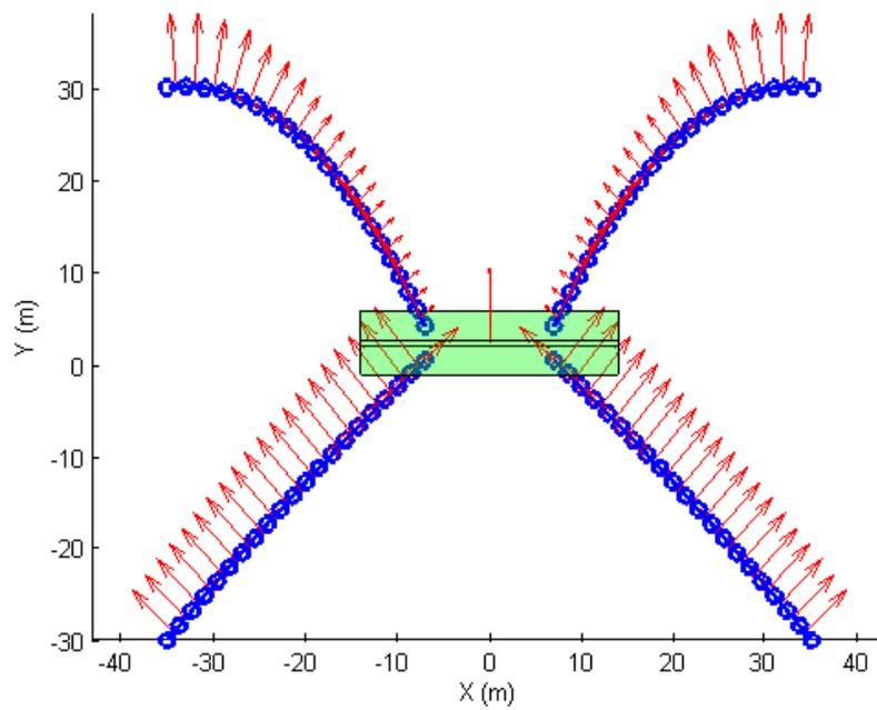
**Figure 5.5** Fourth solution and segment drag forces
