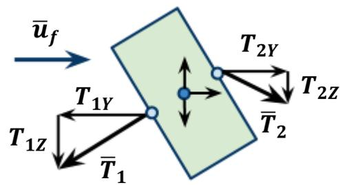
**Figure 5.11** 2D model of tension forces on the body
