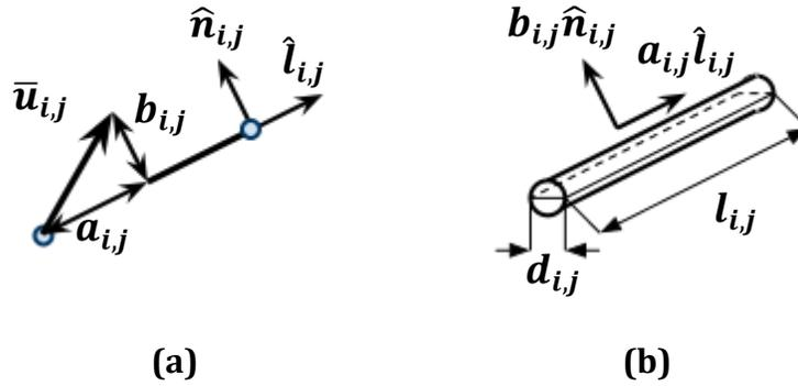
**Figure 3.6 (a)** Segment unit vectors; **(b)** Segment dimensions and relative fluid velocities
