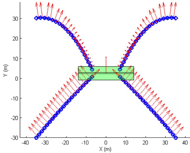
**Figure 5.4** Third solution and segment drag forces
