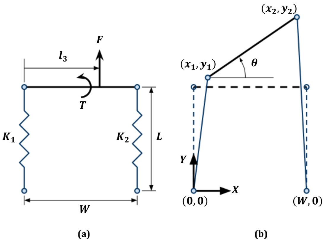
**Figure 4.4** (a) Rigid body test setup; (b) Deformed shape and coordinate system
