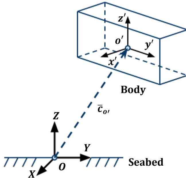
**Figure 2.1** Inertial and body-fixed coordinate systems
