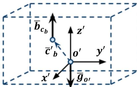
**Figure 3.2** Gravity and buoyant forces on the body
