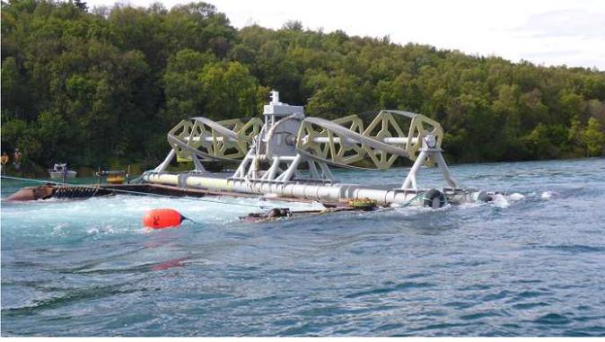
Fig. 1. RivGen turbine generator unit prior to deployment in Kvichak River near Igiugig, Alaska
