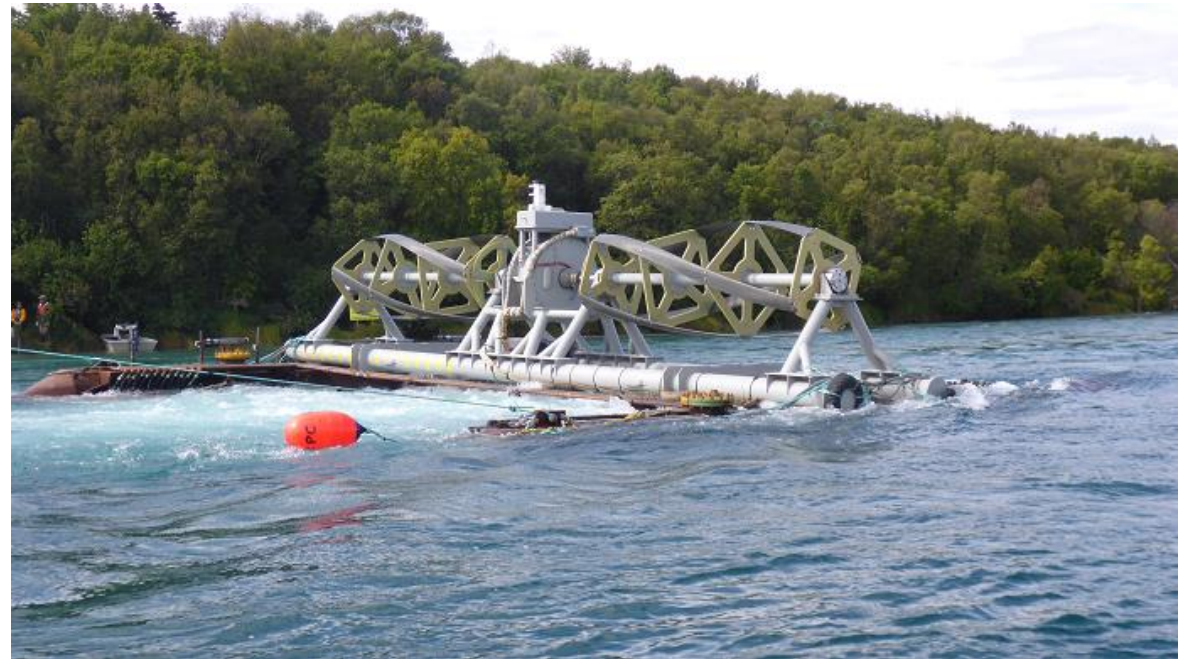
ORPC RivGen cross-flow turbine
