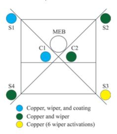
the wiper to automatically actuate, and since the system was power cycled on six occasions, the results for this optical port cannot be considered a control case.
