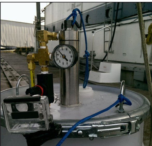
Fig A.3: View of GoPro positioning on the buoy lid
