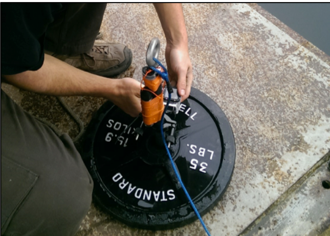
Fig. A.2: Heave plate instrumentation setup
