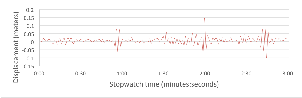
Fig. A.4. Displacement of the buoy for the first three minutes of the lake test
