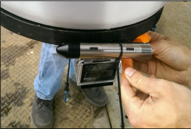
Fig. A.1: Instrumentation attached to underside of buoy.
