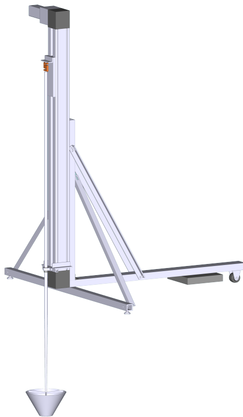
Figure 1: The oscillator measures heave plate position, and the force needed to drive the heave plate. The data is used to calculate phase-resolved hydrodynamic coefficients for the heave plate.
