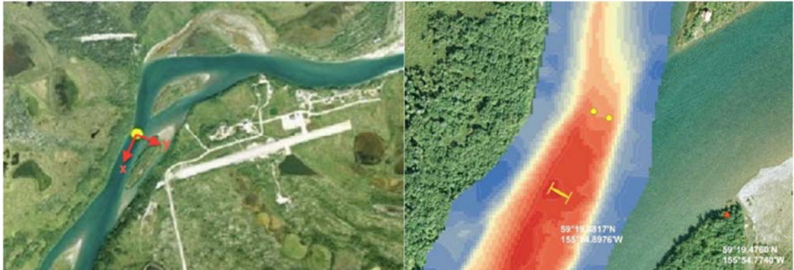
Figure 3: RivGen Site. The village of Igiuig on the Kviachak River, flowing from Lake Iliamna (left, out of frame). The turbine location and coordinate system are shown with satellite view of the village of Igiugig (left). Local bathymetry and locations of upstream anchors can be seen (right). Position of turbine is approximate.
