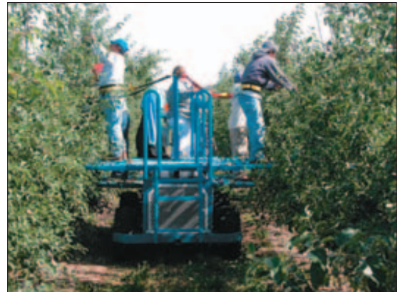
PLATFORM PICKERS: Using platforms, instead of ladders, is one way the tree fruit industry hopes to reduce accidents.
