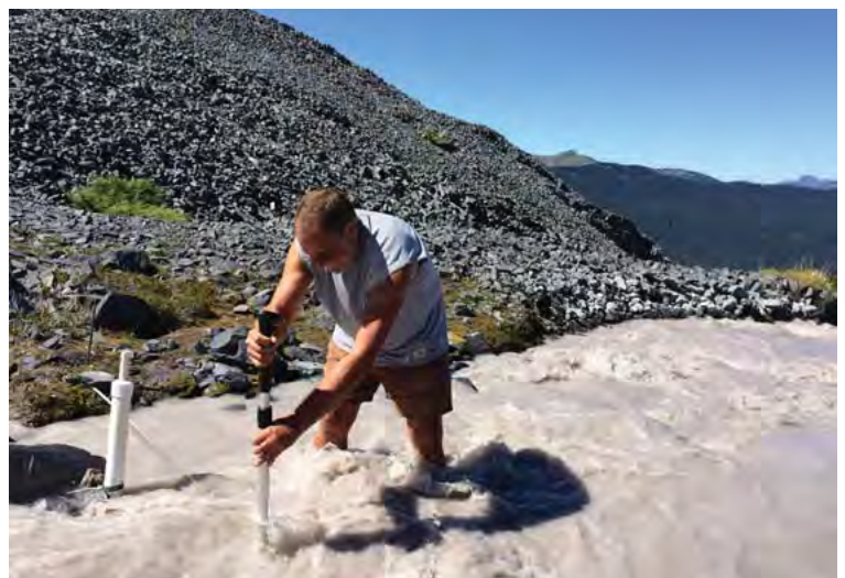
Oliver Grah measures stream velocity as part of the Nooksack Tribe’s glacier monitoring efforts. (Photo courtesy of Oliver Grah, Nooksack Indian Tribe.)
