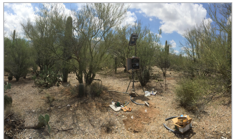
Figure 2. Experimental site where heat dissipation sensors were deployed in July 2015. Focal nurse paloverde is off center with shrubs and a small saguaro located underneath its canopy. Data logger, framing, and solar panel are to the right of the focal individuals. Disturbed soil in the foreground indicate where sensors were deployed away from the nurse for comparison.
