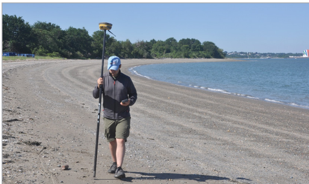
Endicott strolls the beach using survey-grade GPS gear to record precise elevation measurements of coastal features.
