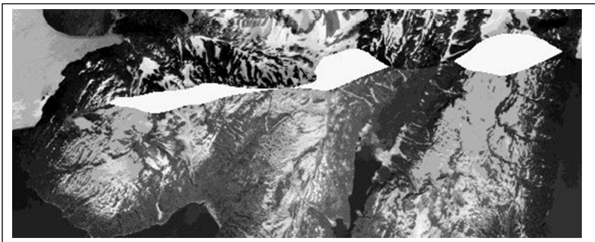
Figure 15. Missing data (white) resulting from poor overlap between adjacent photos.
