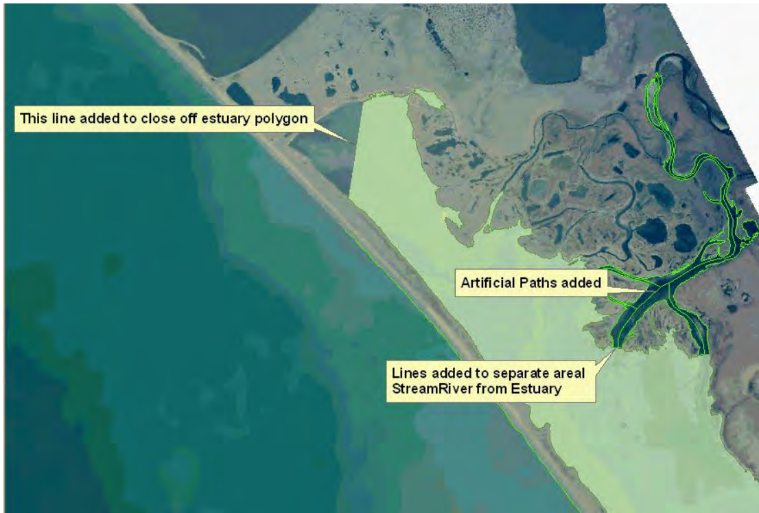
Figure 46. Editing examples. Closing the estuary polygon was necessary because clipping the data to the park boundary, “opened” what would have been a closed polygon. Separation of the StreamRiver from the Estuary is required because once converted to polygon data, the areal StreamRiver will be migrated to the NHDArea feature class while the Estuary will be migrated to the NHDWaterbody feature class. The Artificial Paths are added for inclusion in the NHDFlowline feature class.
