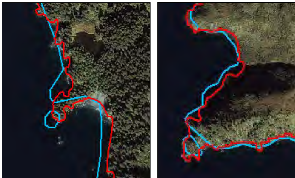
Figure 39. The image series above illustrates how the acceptance of NOAA shoreline data may impact National Map NHD island/islet feature data. In the left-hand image, NOAA EVS data (red) intersects a National Map NHD island feature (blue) near Tooth Cove at KEFJ. In the right-hand image NOAA EVS data encompasses a National Map NHD island feature.
