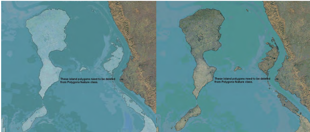
Figure 49. Polygon removal example. Left graphic shows data before the island polygons are removed. Right hand side shows the result after the islands polygons are deleted. Polygons are symbolized in blue with 50% transparency.
