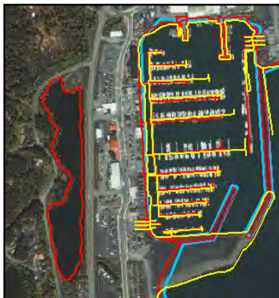
Figure 34. The images series to the left illustrates how EVS data provided by NGS NOAA (red) depicts the MHW level of features that are completely internal to the coast.
