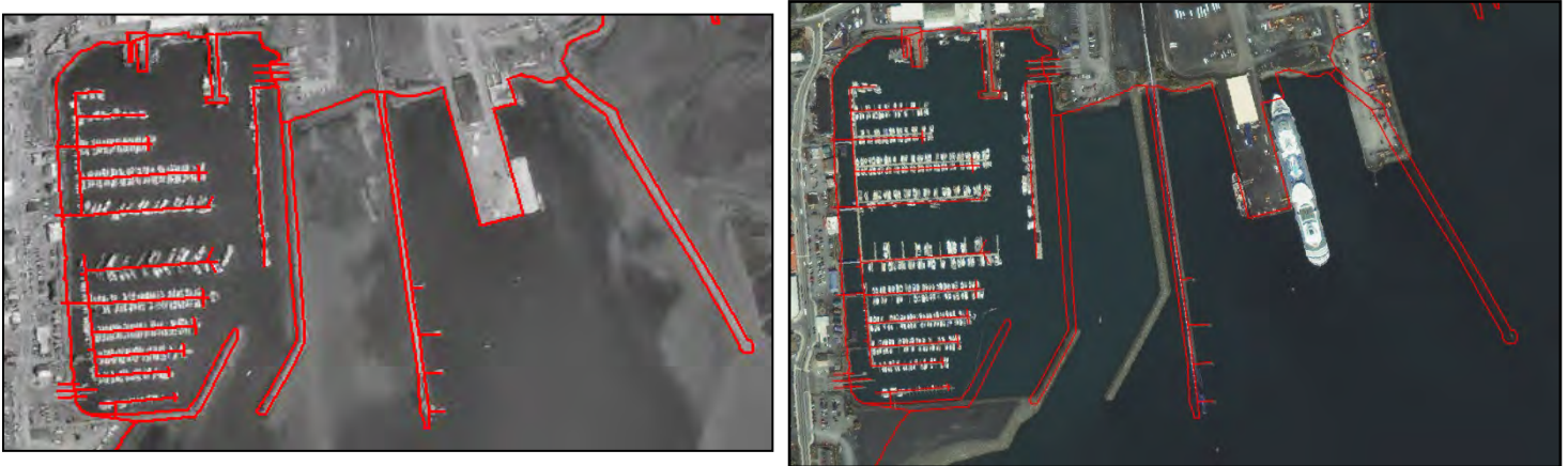
Figure 14. Example of outdated EVS data at the Seward Harbor near KEFJ. The EVS data for this area (red) is derived from survey work conducted in 1992. The linework is consistent with the appearance of the Seward Harbor as seen in the USGS digital orthophoto quadrangle (DOQ) from June 1997 (left), but does not reflect the more recent changes in breakwater or wharf configuration as seen in the 2005 IKONOS satellite imagery (right).
