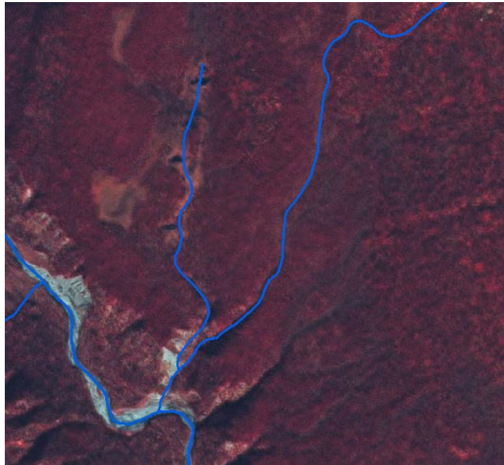
Edited NHD – linears added in correct locations. Contour lines on DRG support these edits as well.
