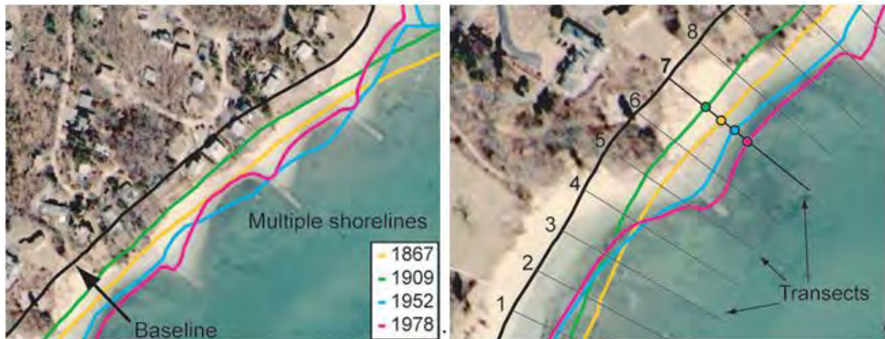
Figure 60. Example of shoreline inputs (left) and resulting transects (right) from the Digital Shoreline Analysis System (DSAS) (Thieler et al. 2009).
