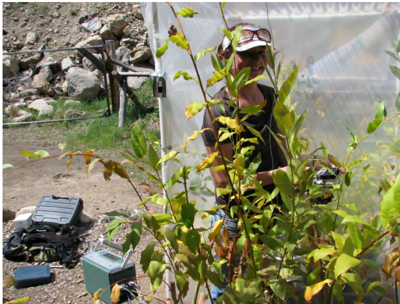
Figure 5: Measuring stomatal conductance and photosynthetic capacity using LiCor 6400XT.
