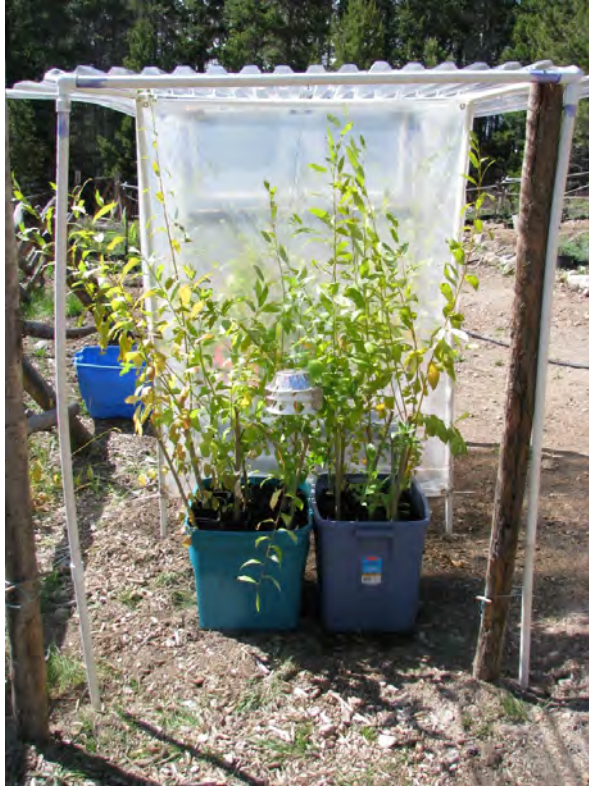
Figure 6: One replication of paired experimental treatments: Ambient temperature in front, warming shelter in plastic sheeting, behind
