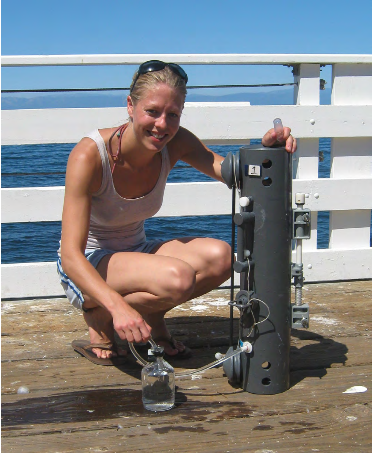
Lydia Kapsenberg collecting a seawater sample using a Niskin bottle, at Santa Cruz Island. These seawater samples are used to calibrate the SeaFET pH sensor (photo by Calla Martyn).
