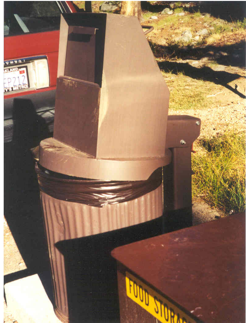
Figure 15. Mailbox-drop system on a dumpster and trash can in Yosemite Valley, Yosemite National Park, California.
