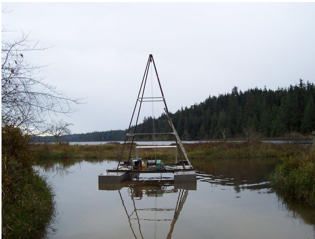
Figure 9. Coring platform constructed to collect sediment cores from Lake Ozette.
