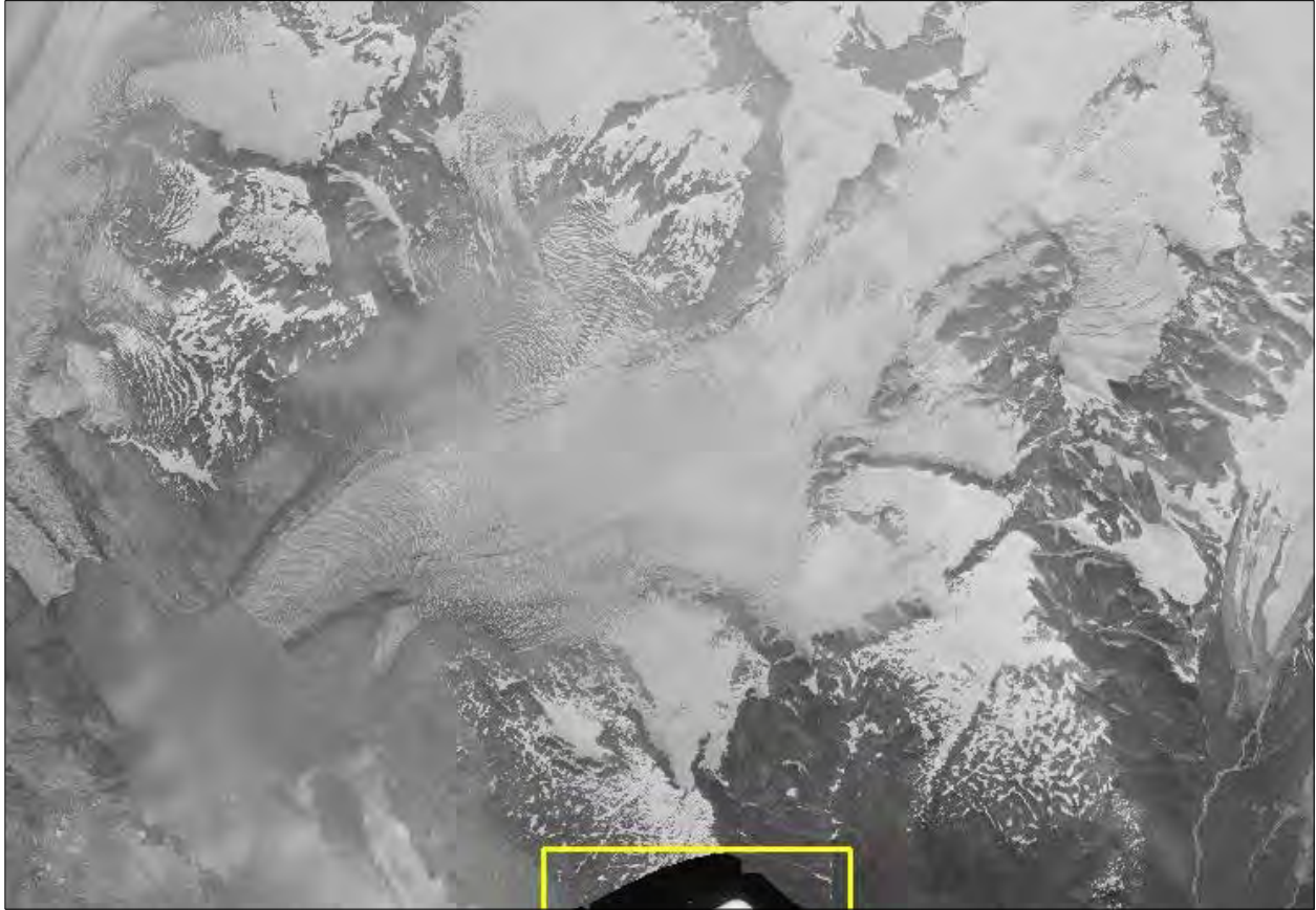
Figure 41. Example of an ortho where the nadir (ortho center), exhibited the least amount of distortion. Northeastern Glacier AOI, KEFJ, B/W, 1950 photograph. Note yellow box and black area at the center bottom of this image (black area) which indicates a gap in the imagery.
