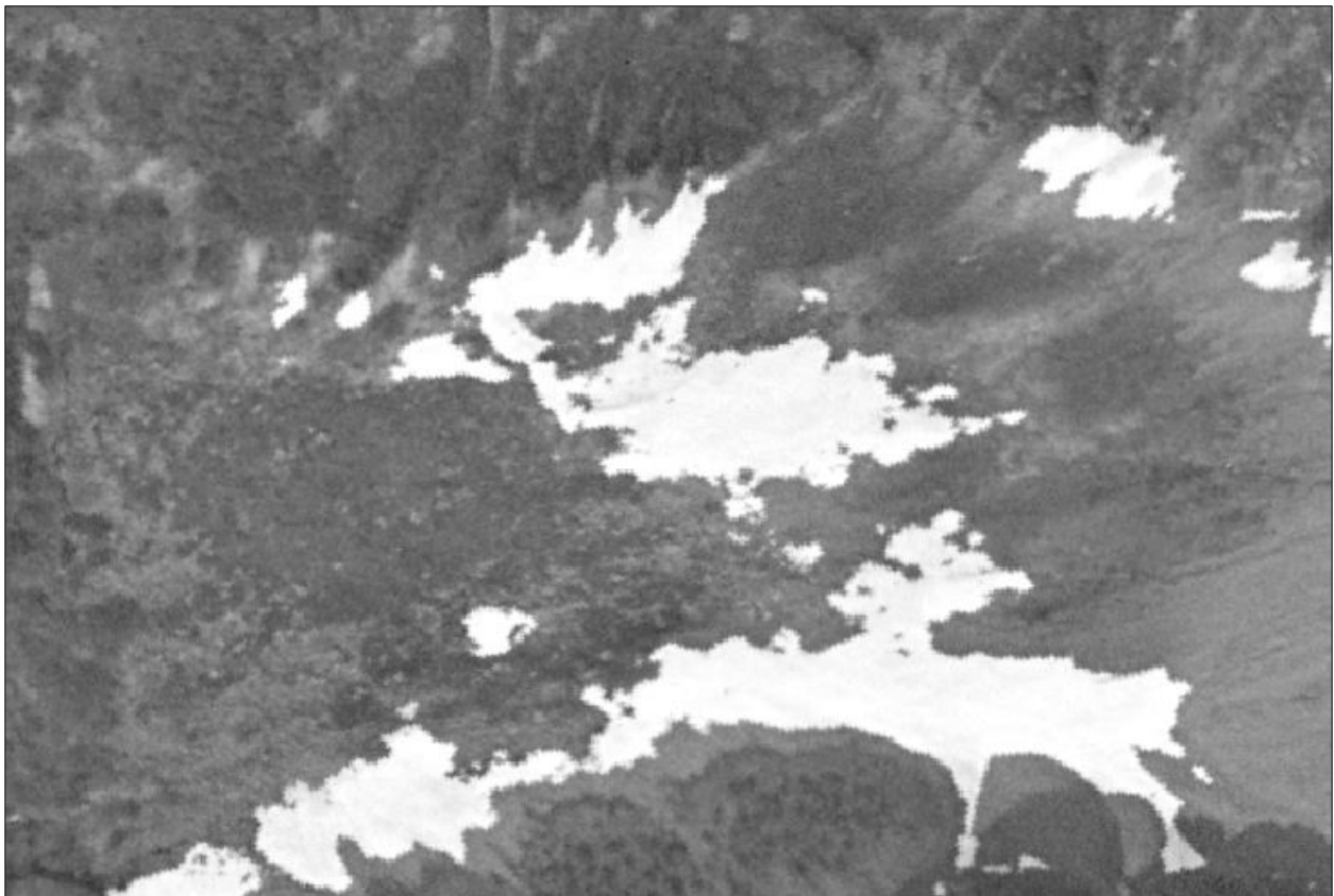
Figure 32. Example of emulsion, Aialik RS AOI, KEFJ, 1950 B/W imagery. Land cover signatures are more difficult to interpret with this type of imagery.
