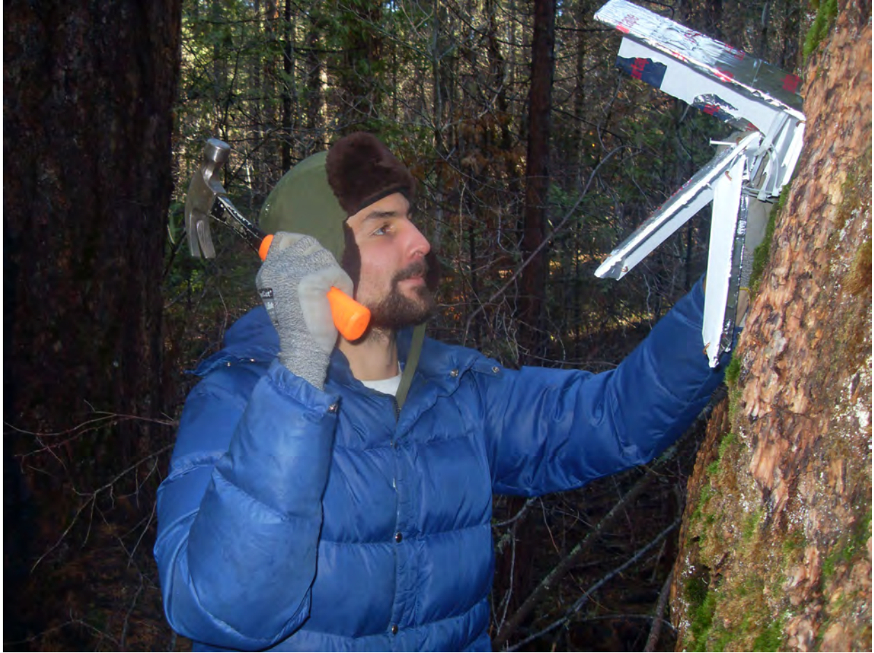
Thomas Reyes attaches a solar radiation shield for the climate sensor network. SDC11786.JPG
