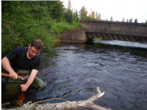
Patrick deploying a temperature logger in the Namekagon River near the USGS gauge at Leonards School Road, Cable, WI.
