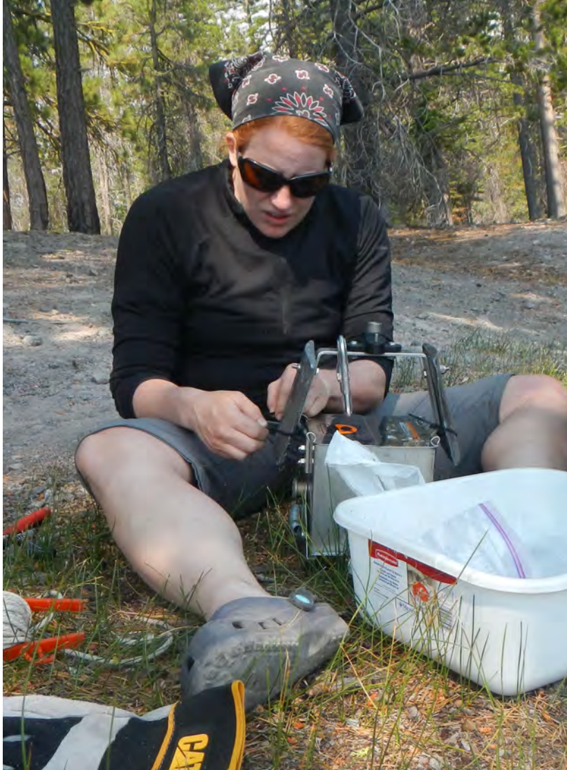
Preparing a sediment grab sampler (Ekman sampler) for use in Manzanita Lake
