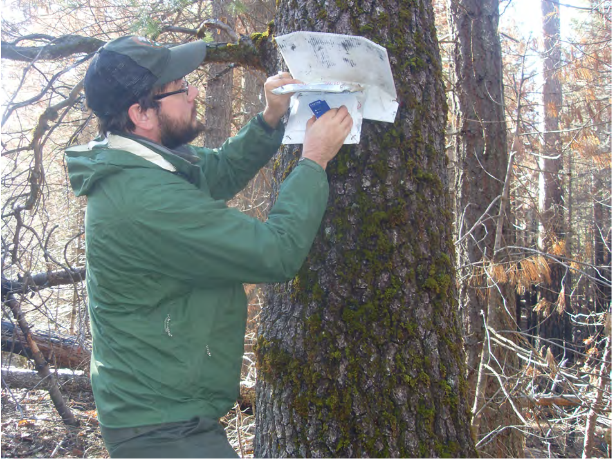
David Campbell places a LogTag climate sensor into a solar radiation shield. SDC11790.JPG
