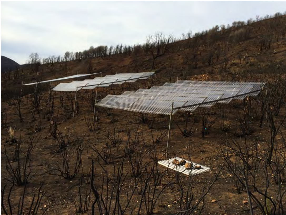
Figure 2. Image of rainout shelters. Flat roofed shelter (far left) excluded 100% of wet season precipitation. Shelters with angled roof panels (center & far right) allowed ambient rainfall to fall on the plots.
