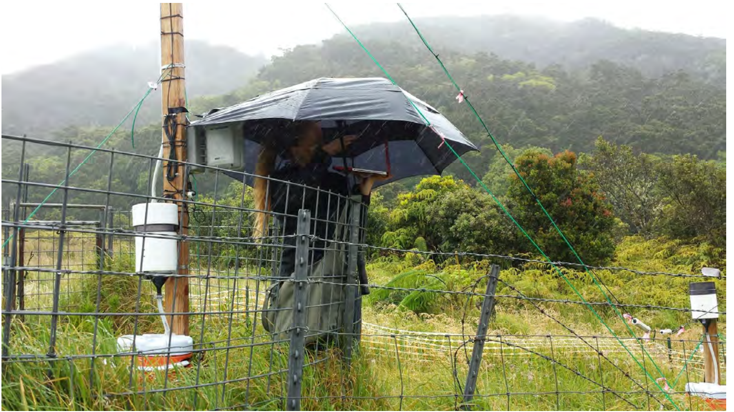
Downloading Data from Climate Station
