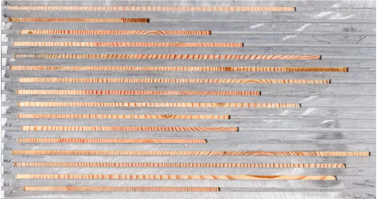
Increment cores collected from conifers in Yosemite National Park. The cores are mounted, sanded, and ready for measuring.
