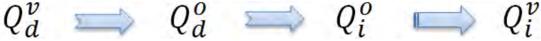
Figure 9. Flow diagram of transforming VIC simulated daily streamflows ( Q_d^v ) into instantaneous ( Q_i^v ) streamflows based on observed daily and instantaneous streamflow ( Q_d^o and Q_i^o ) relationships.
