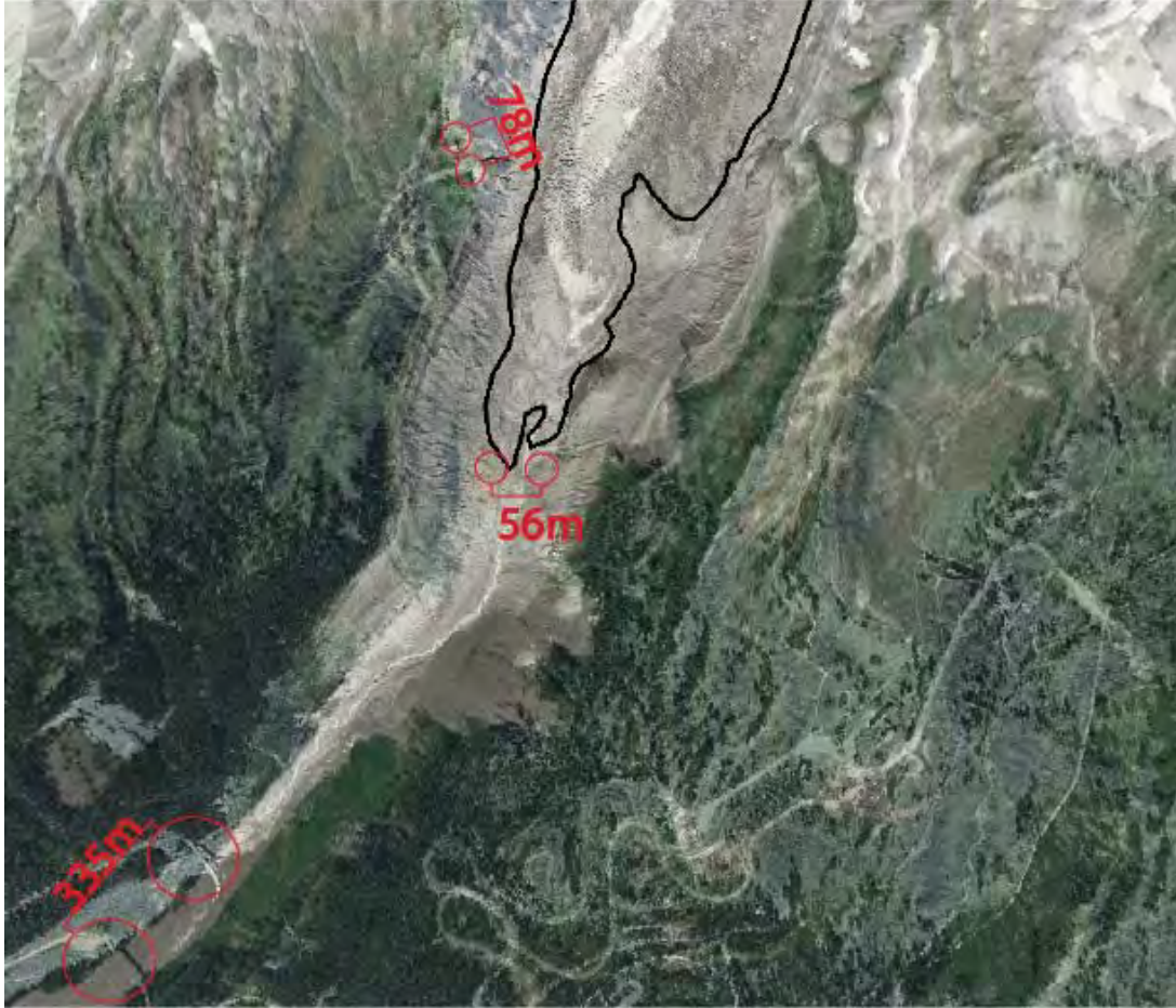
Figure 6: 2013 NAIP and 1951 aerial imagery overlay highlighting georeferencing concerns with regard to image scale inconsistency. These inconsistencies can lead to increased error when using these images to digitize glacier extent and length.
