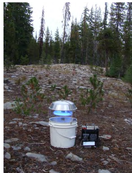
Figure 2. Black light trap used to conduct nocturnal sampling.
