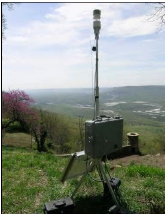
Figure 53. Portable ozone monitor at Lookout Mountain within CHCH (NPS photo).
