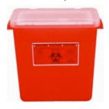
When no more than two-thirds full, close lid and place autoclave tape over lid and sides. Do not block vent holes.
