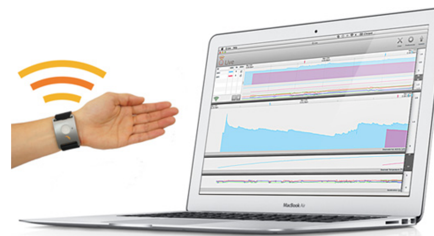
Figure 2: Wireless sensor that measures emotional arousal.
